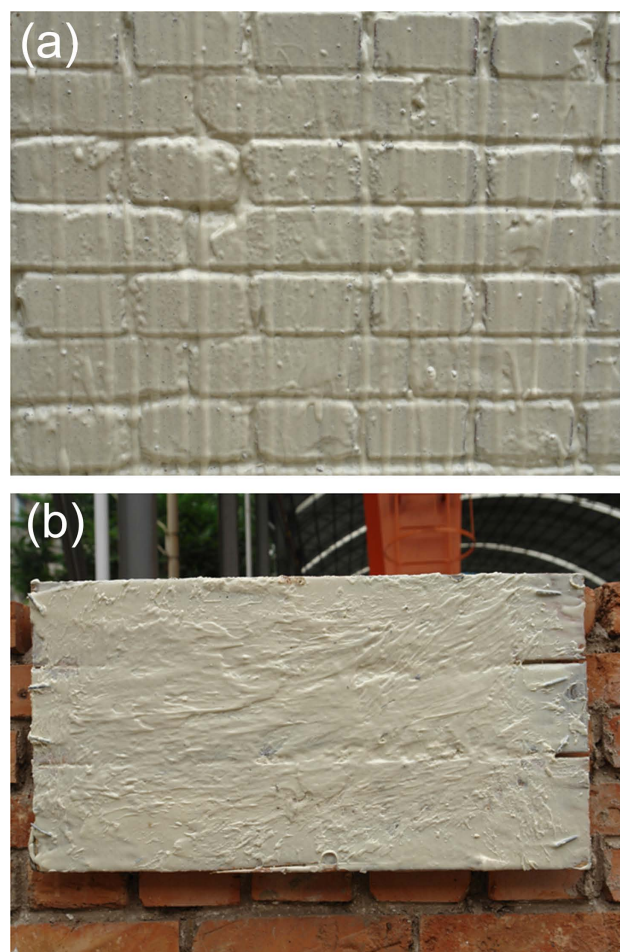
Figure 6. Photographs of PUE in operation with flexible thickness (a) thin coating and (b) thick coating. [Color figure can be viewed in the online issue, which is available at wileyonlinelibrary.com .]
